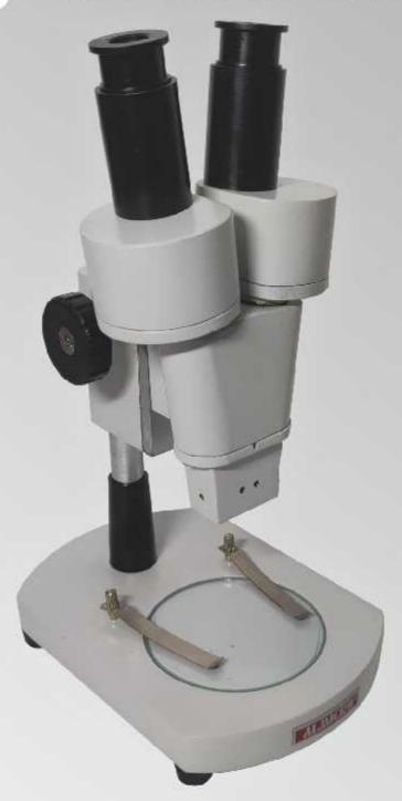
ALMICRO Student stereo Microscope has been designed for Dissection / Inspection of specimens in Biology. Precisely designed long working distance objectives & wide field eyepieces produce an extremely large, brilliant& bright images. It is light in weight having sturdy base, stage with clips and reversible black & white plate, straight Binocular Head with interpupillary adjustment & Hand grip on stand for safe handling.
