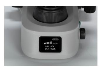
The EXL has a front LCD display, which displays the current lighting brightness, color temperature and magnification, so that the user can Intuitively judge the working status and improve working efficiency.
