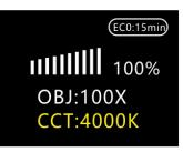
Long press the dimming hand wheel to adjust the color temperature interface 3000K-7000K
